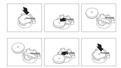
**Note:** Do not bend the top contact tab of the battery holder as it might not make connection with the battery.
