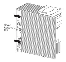
Unlock cover from back of the system unit before removing cover.
