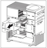
**Note:** The baffle must be installed for proper air flow to the microprocessor(s).
