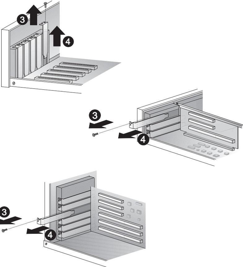
**Figure 2-3. Removing the Expansion Plate**
