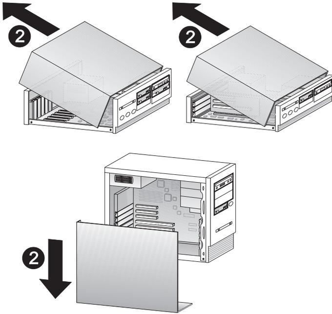
**Figure 2-2. Removing the Computer Cover**
