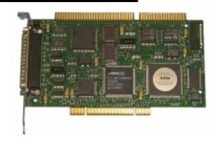
ARTIC is an acronym for A Realtime Interface Coprocessor. The ARTIC family of general-purpose coprocessor adapters can off-load realtime demands, facilitate high-speed communication tasks, and provide front-end processing for a variety of communications data.
