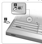
Secure the battery pack by sliding the battery-pack latch to the lock position (3).
