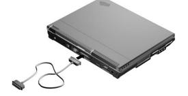
3. Connect the AC Adapter to the computer's power jack (at the rear of the computer) in the order shown.
