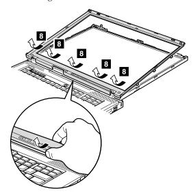
When installing: Attach the LCD cover kit as follows:
