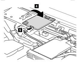
**When installing:** Make sure that the modem connector and the connector on the underside of the card are attached firmly.
