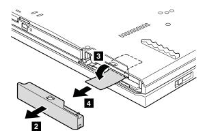
When installing: Make sure that the hard disk drive connector is attached firmly.
