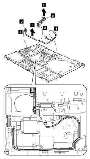
**When installing:** Make sure the connectors are attached firmly, and that the cables are routed as in the figure above.
