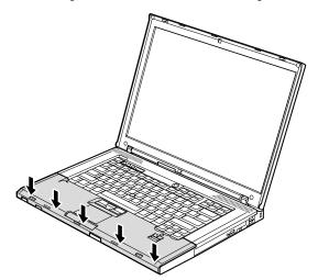
4. Close the LCD cover and turn the computer over. Then fasten the four screws to secure the palm rest.
