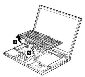
**When installing:** Make sure that the keyboard edges a are under the frame as shown in this figure.
