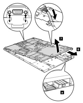
Remove the USB sub card with cable and the security hole bracket as in this figure.
