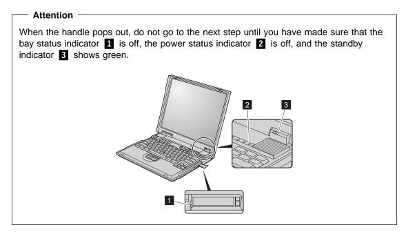
$m{2}$  Pull the handle until it stops  $m{2}$ ; then pull out the Ultrabay 2000 device  $m{3}$ .
