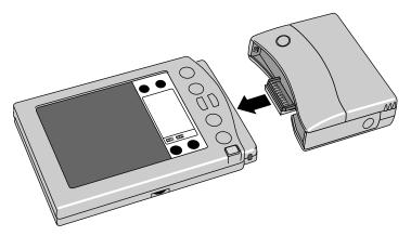
When correctly installed, the curved edge on the bottom of the WorkPad aligns smoothly with the modem.
