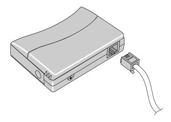
2. Insert the other end of the cable into an analog telephone jack on the wall.
