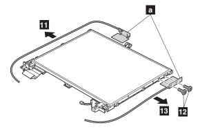
Remove the hinges ( b ) from the LCD assembly.
