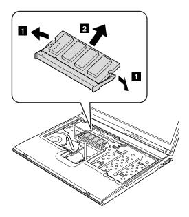
When installing: Insert the notched end of the DIMM into the socket. Press the DIMM firmly, and pivot it until it snaps into the place. Make sure that it is firmly fixed in the slot and does not move easily.
