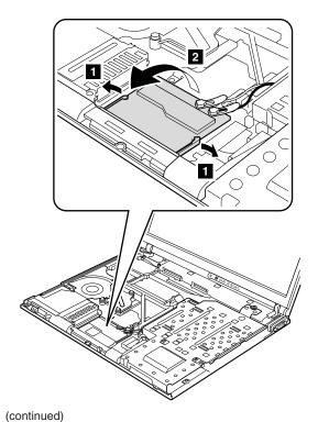
If the wireless antenna jacks have tabs marked "MAIN" or "AUX", unplug the jacks by pulling the tabs with your fingers. If the antenna jacks do not have the tabs, unplug the jacks by using the removal tool antenna RF connector (P/N: 08K7159) or pick the connectors with your fingers and gently unplug it in direction of the arrow 3.
