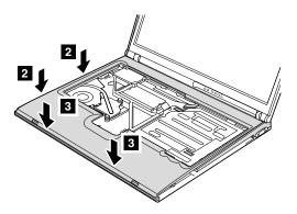
3. Secure the keyboard bezel from the underside of the computer with the screws.
