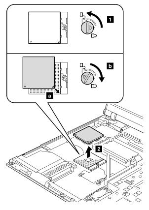
When installing: Place the CPU on the CPU socket a, and then rotate the head of the screw in the direction of arrow b to secure the CPU.
