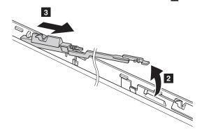
When installing: Attach the left latch to the LCD cover as in this figure.
