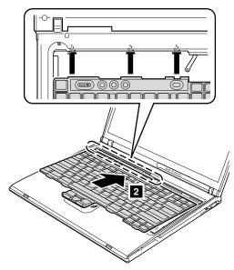
To make sure that the front edge of the keyboard is housed firmly, gently press the keys with your fingers and try to slide the keyboard towards you.
