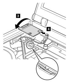
When installing: Make sure that connector 4 and the connector on the underside of the card are firmly attached. Then place the cable to fit in the cable guide as in the figure.
