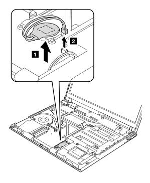
When installing: Make sure that the battery connector 2 is firmly attached.
