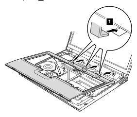
While inserting the three latches, align the top-left corner of the keyboard bezel as in figure a.
