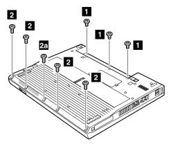
Screw 2a is only for the models with 15.0-in. LCD.
