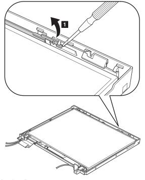
Lift the latch bar in the direction of the arrow 2, and then remove the left latch in the direction of the arrow 3.
