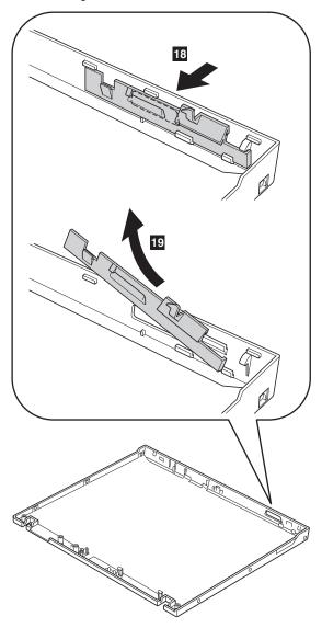
When installing: Attach the right latch to the LCD cover as in this figure.
