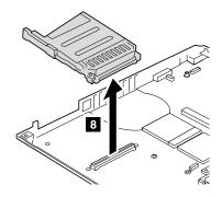
When installing: Make sure that the connector 8 is firmly attached to the system board. Then, secure the screws from the underside of the computer.
