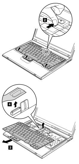
When installing: Make sure that the connector 4 is firmly attached.
