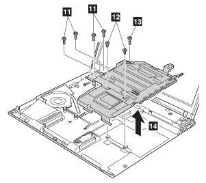
Screws 11 are only for the models with 15.0-in. LCD. For the other models, skip the step.
