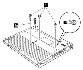
Screw 1a is only for the models with 14.1-in. LCD.
