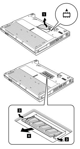
When installing: Insert the notched end of the DIMM into the socket. Press the DIMM firmly, and pivot it until it snaps into the place. Make sure that it is firmly fixed in the slot and does not move easily.
