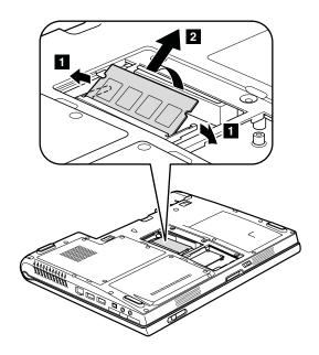
When installing: Insert the notched end of the DIMM into the socket. Press the DIMM firmly, and pivot it until it snaps into the place. Make sure that it is firmly fixed in the slot and does not move easily.
