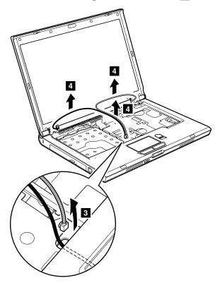
When installing: Route the antenna cables along the cable guides. When you route the cables, do not tense them. To do so, the cables may get damaged by the cable guides of the frame, and may cause a broken wire.
