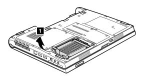
When installing: Make sure that the hard disk drive connector is attached firmly.
