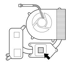
When installing: Before you attach a new heat sink assembly to the computer, peel off the covering film of thermal grease. Then attach the heat sink assembly to the computer.
