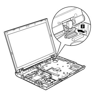
When installing: Make sure that the connector is attached firmly.
