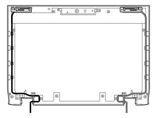
For the antennas with three cables
