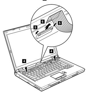
When installing: Make sure that the connector is attached firmly.
