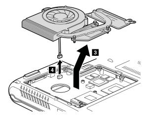
When installing: Make sure that the fan connector is attached firmly.
