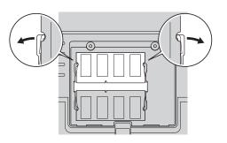
**9.** Replace the memory slot cover by aligning the back side of the cover first and then tightening the screws.
