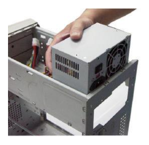
1. The power supply should be installed in the back of the chassis. This is to draw the air out of the inside of the case. Check the position of the power supply fan as shown in the figure.
