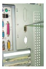
**5**. Remove one screw from the USB bracket using a screwdriver.
