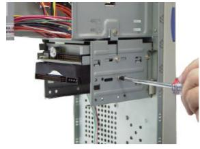
Always secure the screws when installing the drives. This will prevent them from moving and falling from the storage bay.
