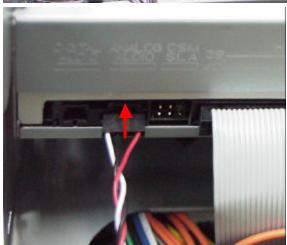
17. Then attach the other end of the cable to the CD-ROM drive audio port.
