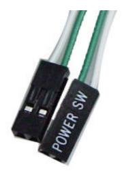
1. Connect the Power LED and Power SW cable on the Panel 1 of the mainboard. The Power button located in front of the case only works when the Power Switch connector is connected to the mainboard.
