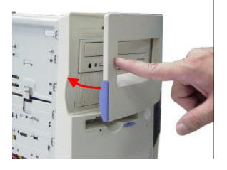
**7**.Close the door panel. This completes the setup for the CD-ROM drive.
