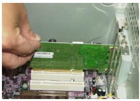
**5**.Next, install the Modem card as the same way with the AGP card. Insert the Modem card to the first 32-bit PCI slot. Refer to the figure for reference.
