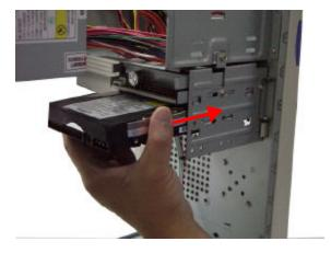
3. For the hard disk drive, follow the same manner for installing the floppy disk drive.
