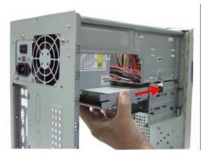
1. There are two different size "bays" into which each of the various drives will fit. Take a close look at the drive and determine which is the "bay" for the floppy drive. Install the floppy drive into the upper side of the storage bay. See figure for reference.
