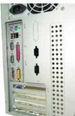
2. Remove the dust cover from the COM port as shown in the figure.
