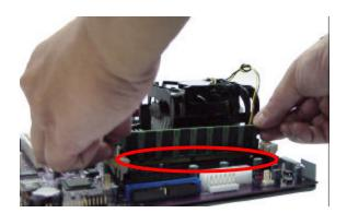
**9**.Open the left and right levers of the slot. Then firmly slide the Memory Module into the DIMM slot. The DIMM slots are keyed with notches and the DIMMs are indicated with cut outs so that they can only be installed correctly.
