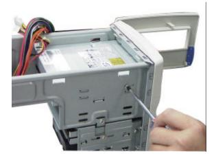
**6**. When the CD-ROM drive is positioned correctly, secure the drive to the bay using four screws.
