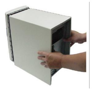
3. Using both hands, gently pull back the top cover as shown in the figure. Slide the cover up off the frame of the case.
