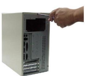
**2**.Locate the 3 screws at the back of the case; use the screwdriver to loosen them.
