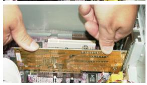
**3**.Using both hands, gently press down the AGP card firmly to ensure that the edge connector is correctly rested in the slot.
