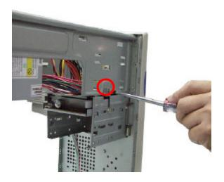
1. After you have installed the mainboard into the case, you should connect the power cable from the case power supply unit to the mainboard power connector. Since the floppy drive is situated closely to the power supply. For convenience purpose, loosen the screw that holds the Floppy drive.
