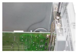
7. Secure the metal bracket of the Modem card with a screw.
