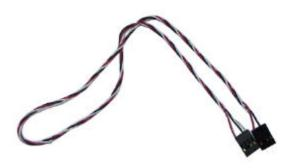
15. Use the audio cable provided with the CD-ROM drive to connect the audio connector on the rear edge of the CD-ROM drive to one of the audio-in connectors on the mainboard. The audio sound does not come from the mainboard itself.
