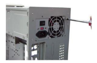
2. Using the screwdriver, gently tighten the three screws.
