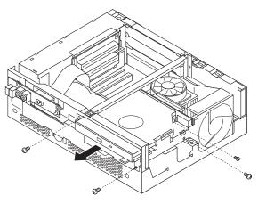
7. Due to cable length limitations both drive trays must slide outward together. Slide both drive trays out far enough to access the system board. This might require disconnecting cables that are connected to the drives and to the system board. Note where the cables are connected before disconnecting them.
