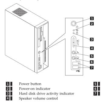
Headphone connector Microphone connector USB connectors
