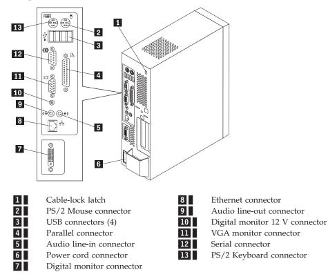
**Note:** Some connectors on the rear of your computer are color-coded to help determine where to connect the cables.
