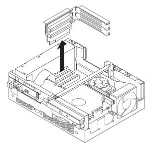
**3**. Remove the adapter-slot-cover latch and the slot cover for the appropriate expansion slot.
