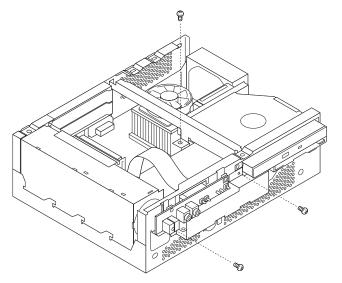
5. Unplug the flat cable attached to the small circuit board at the front.
