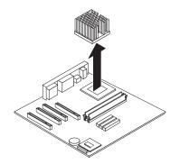
5. To remove the fansink from the processor twist the fansink to break the seal formed by the thermal grease and remove.
