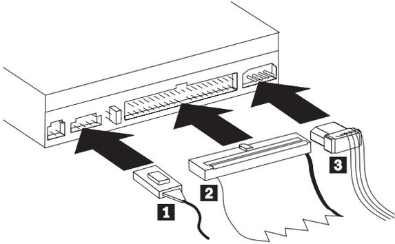
1. If you have an audio adapter, locate the included audio cables and determine which cable best fits the CD audio-in port on your audio adapter. Connect one end of the selected audio cable to the device audio-out connector **1**, and the other end of the cable to your audio adapter CD audio-in port. Save the other cable in case you use a different audio adapter in the future.
