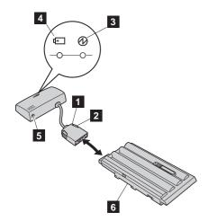
1. The **connector** for connecting the battery charger to the battery pack for ThinkPad i Series 1200 and 1300
