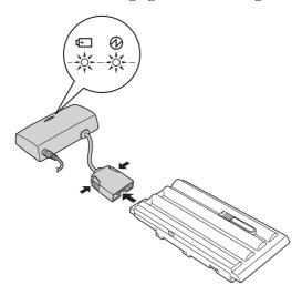
4. When the charging indicator turns off, the battery pack is fully charged.
