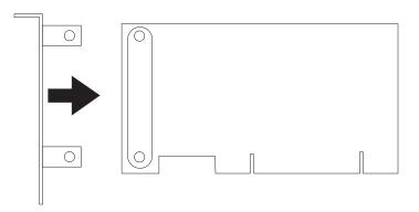
d. Insert the two screws **1** and carefully tighten the screws. Do not overtighten.
