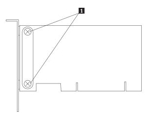
e. To verify that the bracket is correctly installed, be sure that the bent or L-shaped part of the bracket is near the edge *opposite* the adapter contacts. The screw heads rest against the component side of the adapter and the bracket rests against the *opposite* side.
