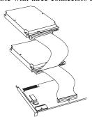
Connect one end of the IDE cable to the IDE port, and connect the other end to a storage device. You can attach an additional storage device to the middle connector. The IDE port can be on the computer system board or on an adapter installed in an expansion slot. For the best signal quality when you have only one device on the IDE cable, connect the device to the connector on the end opposite the IDE port.
