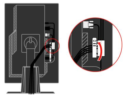
Wrap the Cable Wapper around the cables.
