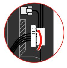
Wrap the Cable Wapper around the cables.
