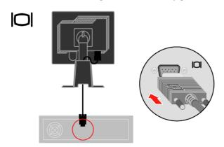
Connect the digital cable to the DVI connector of the monitor and the other end on the back of the computer.
