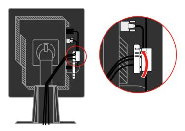
Wrap the Cable Wapper around the cables.
