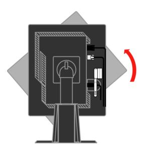
Place the cables through the Main Clip. Then fasten the clip.
