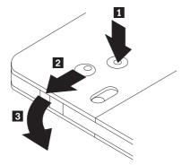
Using the tip of a ballpoint pen, push and break the lock pin tab 1. To remove the disc, use a ballpoint pen to push down on the cartridge-lid lock 2 and pull the cartridge lid 3 out to eject the disc. With the cartridge lid open, the disc will eject.
