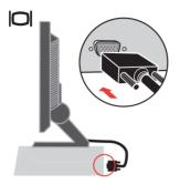
3. Insert the power cord into the monitor, then plug the monitor power cord and the computer cord into grounded electrical outlets.
