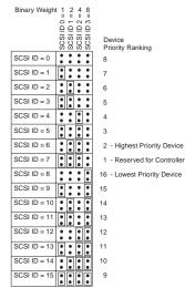
Save any spare jumpers; you might need to change the SCSI ID later. Refer to the *SCSI Hard Disk Drive User's Guide Supplement* to see if you can safely store spare jumpers on the drive jumper pins.
