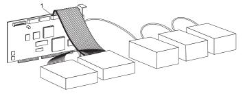
You cannot end the SCSI chain with devices that use passive termination, such as some CD-ROM drives, tape drives, and optical drives.
