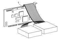
Remove any terminators or terminating jumpers on devices in the middle of the chain.
