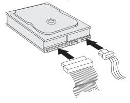
2. Attach an available connector on the SCSI cable to the connector on the hard disk drive, as shown.
