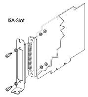
3. Hold the adapter by the top, insert it into the expansion slot, and press it firmly into place.
