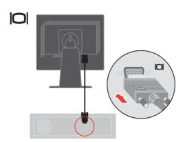
Connect the digital cable to the DVI connector of the monitor and the other end on the back of the computer.
