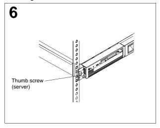
Tighten the thumb screws on the front of the server to secure it to the rack.
