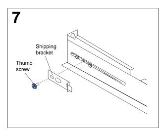
If you want to ship your rack with the server installed, you must install the shipping brackets on each side of the server. This is done by inserting the shipping bracket tab into the slot on the back of the server. Then use the blue thumb screw to secure the back of the server and the shipping bracket to the mounting bracket.
