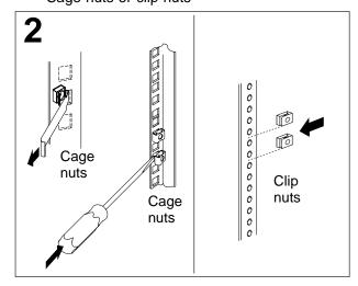
Select a 1 U size location in the rack. Install a cage nut or clip nut in the top and bottom position of the 1 U location you selected (both sides, front and rear of the rack).
