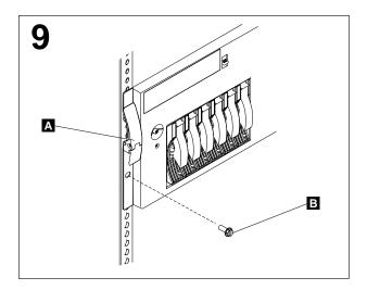
Slide the server into the rack until the release latches A located on the front of the server, snap shut. Then, insert the M6 screws B through the release-latch-bracket assembly.
