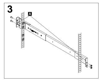
Use the pins **A** on the slide rail to align the slide rail to the rack. Use the M6 screws to bolt the slide rail to the rack. Repeat this step for the other slide rail.
