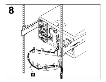
Route all the cables through the cable-management assembly as shown. Then, use the cable straps **A** to secure the cables to the cable-management assembly.
