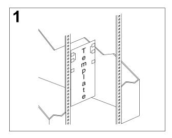
Use the attached stickers to mark the holes on the front and rear of the rack in the locations as indicated by the arrows on the attached template.
