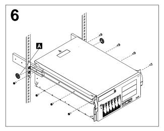
Use the M4 screws to secure the server to the rails. Unscrew the rack-support wheels A and store them for potential future use.
