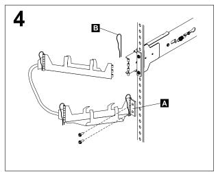
Use the M6 screws to attach the hinge bracket A to the rear of the rack.
