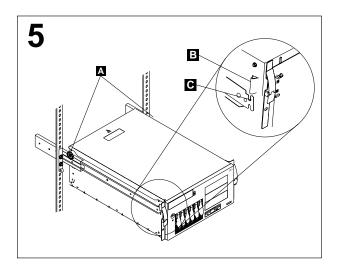
**Caution:** To avoid injury, do not place your fingers around the rack-support wheels when lowering the server onto the rails.
