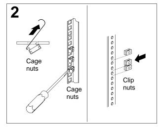
Use the cage-nut-insertion tool or a screwdriver to install the cage nuts, or the clip nuts, as required for your rack, into the marked holes.
