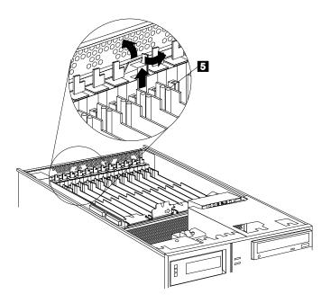
5. If you are installing a hot-plug adapter, disable the PCI slot from your operating system. Make sure that the Power On light for the PCI slot is off. (Refer to the documentation that comes with your operating system for information about disabling a hot-plug PCI slot.)
