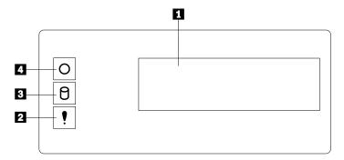
Information message panel: System monitor information appears on this display. The Advanced System Management PCI adapter monitors system functions and generates the messages.
