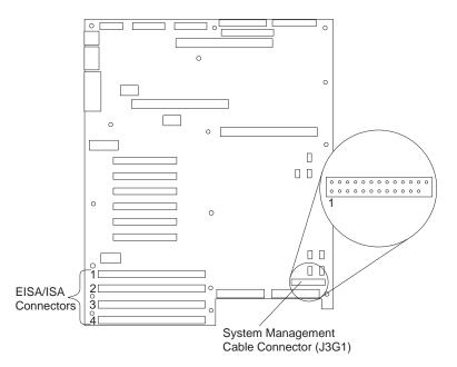
Figure 7. PC Server 704 System Board
