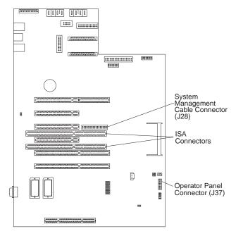
Figure 5. PC Server 330 Models 8640-PB0, PM0, PT0 System Board
