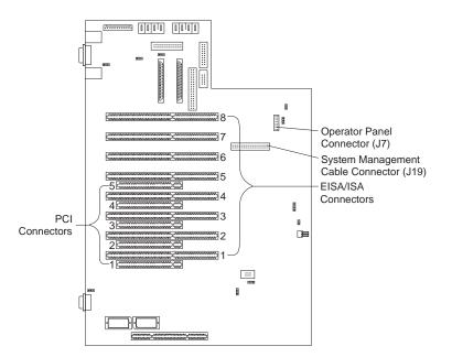
Figure 4. PC Server 330 Models 8640-ES0, ES2, ESS, EM2, EMR System Board
