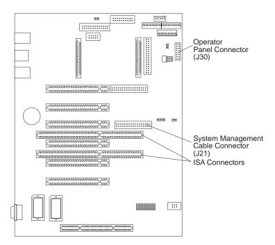
Figure 2. PC Server 325 Models 8639-PB0, PTW, PT0, RB0 System Board
