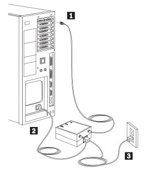
Figure 11. Power Unit Cables
