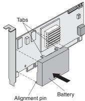
6. Press gently on the *center* of the battery pack to snap the battery pack into place. Be sure to apply pressure evenly with both hands and to hold the controller as shown in the figure below. Also, make sure that the tab is properly latched on the controller.
