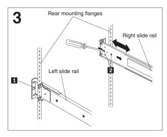
Use the tab 1 on the rear of each slide rail to align the slide rail to the rear mounting flanges. If the front slide rail bracket does not align with the front mounting flange, slightly loosen the rail-length-adjusting screws 2 and adjust the length of the rail.
