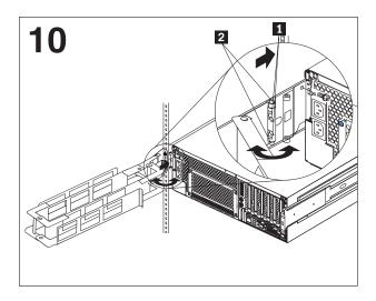
Slide the server fully into the rack cabinet until it locks in place. Using the handles 1 on the free end of the cable management arm, retract the spring-loaded hinge pins 2; then, rotate the handles to lock the pins in the retracted position.
