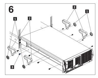
Use four M4 screws per side to secure the server to the rails; then, remove the rack-support wheels 1 and the handles 2 and store them in a safe place. Also remove the blue thumbscrew 3 from the left side of the server and store it in a safe place.
