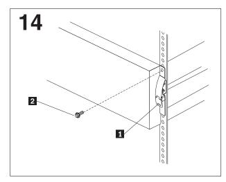
Slide the server into the rack cabinet until the release latches 1 lock into place.
