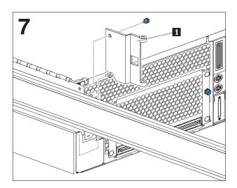
Insert the tab on the bottom edge of the cable management arm hinge plate 1 into the slot at the rear-left side of the server; then, attach the plate to the server with the M3.5 thumbscrew.
