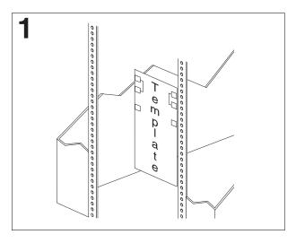
Use the attached rack mounting template to locate the holes on the front and rear rack mounting flanges.
