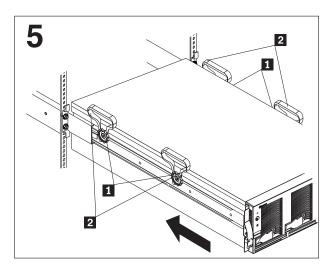
**Attention:** To avoid injury, do not place your fingers around the rack-support wheels **1** when positioning the server on the rails.
