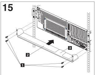
**Important:** The chassis support bracket must be installed if you move the rack cabinet after you install the server.
