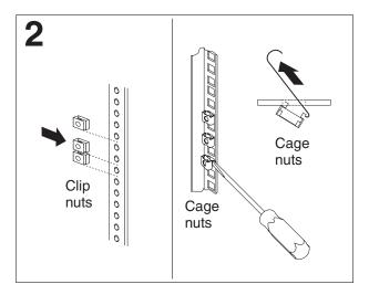
Install cage nuts or clip nuts as required for your rack cabinet. Use the cage-nut-insertion tool or a flat-blade screwdriver to install cage nuts.
