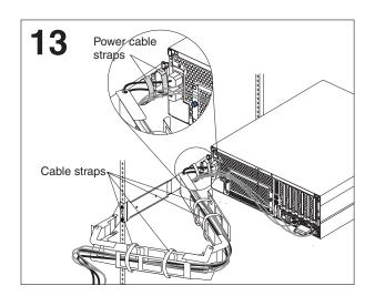
Route the cables through the cable-management arm, securing them with cable straps. Use two cable straps (one on each side of the hinge) to secure the power cords to the hinge plate.
