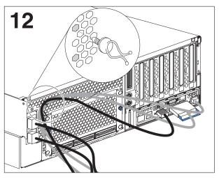
Attach cables to the rear of the server (such as keyboard, mouse, and monitor cables if required). Route the cables toward the left side of the server. Use the cable clamps to secure cables along the way. Insert clamps only in the column of ventilation holes immediately to the right of the ac power connectors. If you insert the clamps in columns elsewhere, they will interfere with the removal of internal components.
