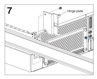
Insert the tab on the bottom edge of the cable-management-arm hinge plate into the slot at the rear-left side of the server; then, attach the plate to the server with the M3.5 thumbscrew.
