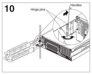
Slide the server fully into the rack cabinet until it locks into place. Using the handles on the free end of the cable-management arm, retract the spring-loaded hinge pins; then, rotate the handles to lock the pins in the retracted position.
