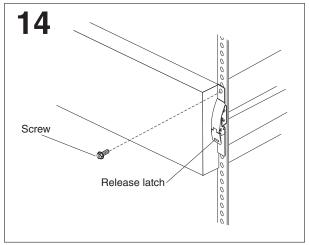
Slide the server into the rack cabinet until the release latches lock into place.
