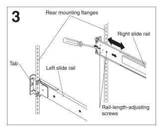
Use the tab on the rear of each slide rail to align the Install the slide rails, ensuring that the front and slide rail to the rear mounting flanges. If the front slide rail bracket does not align with the front mounting flange, slightly loosen the rail-length-adjusting screws and adjust the length of the four front M6 screws. the rail.
