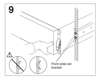
Slide the server halfway out of the rack cabinet; then, loosen but do not remove the four front M6 screws. While one person supports the front of the server by lifting it slightly, ensure that the front slide-rail brackets are vertically aligned; then, fully tighten the four front M6 screws.
