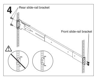
rear slide rail brackets for both slide rails are vertically aligned. Insert and partially tighten the four rear M6 screws; then, insert and fully tighten
