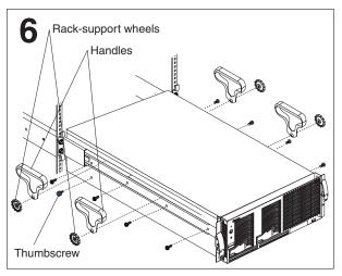
Use four M4 screws per side to secure the server to the rails; then, remove the rack-support wheels and the handles and store them in a safe place. Also remove the blue thumbscrew from the left side of the server and store it in a safe place.
