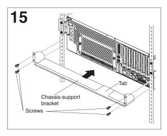
**Important:** The chassis-support bracket must be installed if you move the rack cabinet after you install the server.
