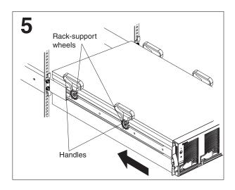
**Attention:** To avoid injury, do not place your fingers around the rack-support wheels when positioning the server on the rails.
