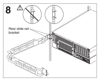
Press in on the slide-rail-locking latches and slide the server fully into the rack cabinet. Slide the cable-management-arm bracket over the right-rear M6 screws. Ensure that both rear slide-rail brackets are vertically aligned; then, fully tighten the four rear M6 screws.
