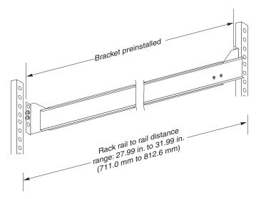
2. Hold a rack-cabinet rail up to the vertical EIA rails of the rack cabinet with the outside of the flanges positioned inside the front and rear EIA rails.
