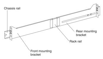
**3**. Rotate the lever on each chassis rail and pull forward to remove the chassis rail from the rack-cabinet rail.
