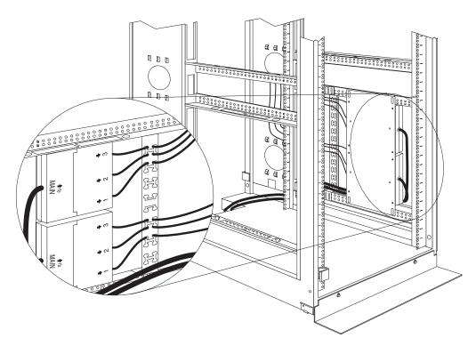
Figure 61. Connecting and routing other power cables to the outlets
