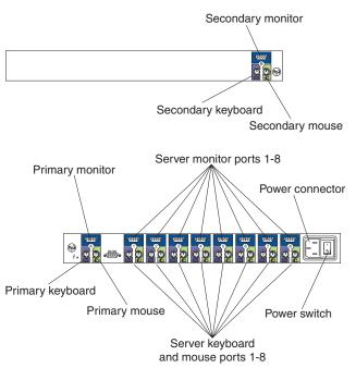
You can connect multiple console switches to each other in a tiered configuration. If you use a 1x4 Console Switch as the primary switch, you can connect up to four additional console switches and 32 servers. If you use a 2x8 Console Switch as the
