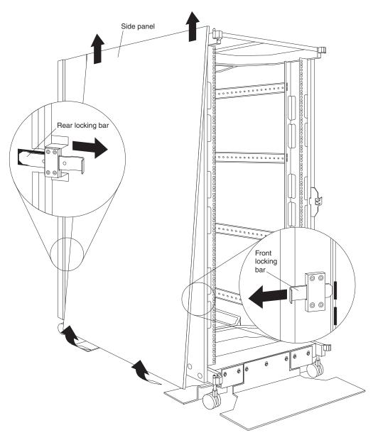
Figure 10. Removing the NetBAY42 side panels
