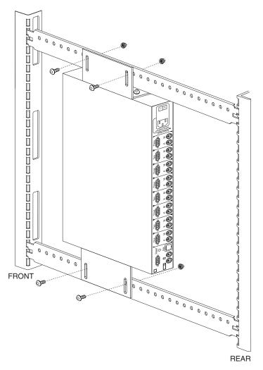
Figure 74. Selector switch between side panels
