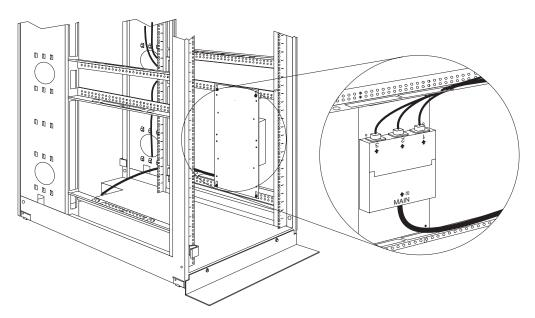
Figure 56. Routing the fixed line cord and power cables
