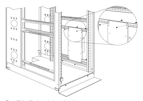
Figure 55. Installing the vertical mounting plate
