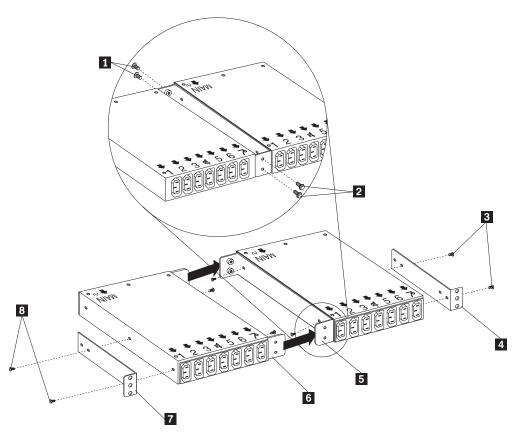
Figure 48. Installing the mounting brackets for two devices
