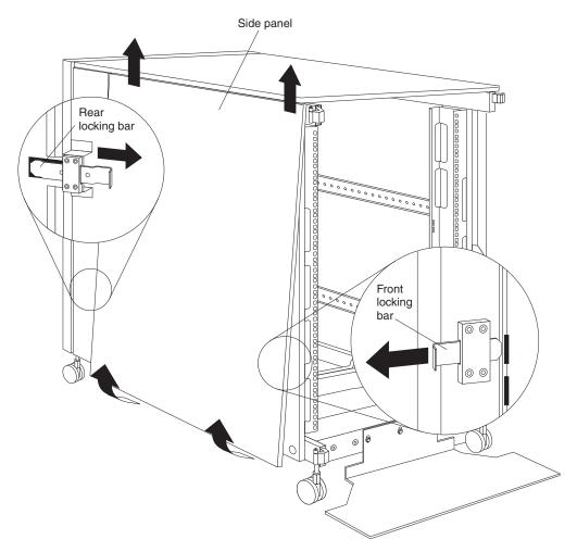
Figure 8. Removing the NetBAY25 side panels
