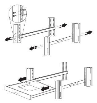
To remove the tray from the side rails, pull up on the left rail tab and push down on the right rail tab.
