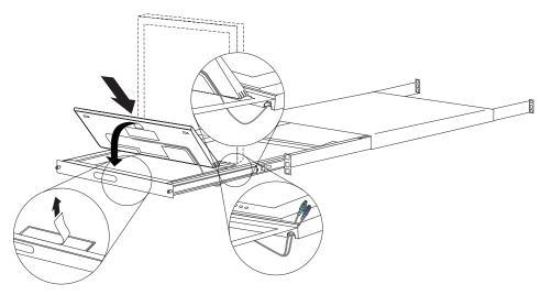
7. To install the keyboard in the tray, align the top slot on the rear of the keyboard with the back edge of the large rectangular opening in the front of the tray; then, carefully rotate the front of the keyboard down and into the tray.
