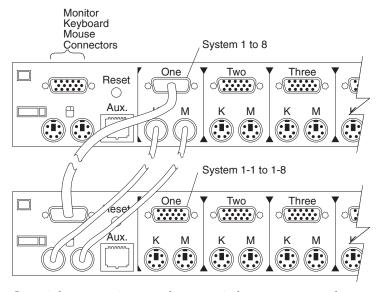
One eight-port primary selector switch can accommodate up to eight secondary selector switches which can then support up to 64 servers.
