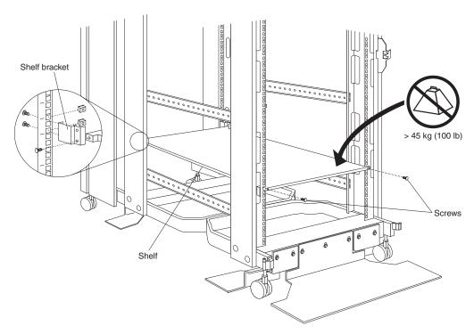
Figure 37. Installing a fixed shelf
