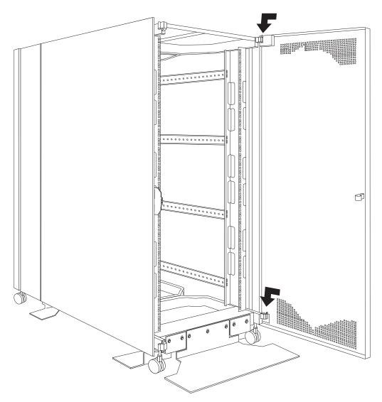
Figure 15. Rotating and installing the door
