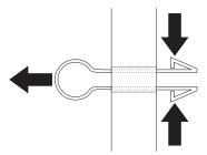
Figure 79. Removing the plastic cable clamp
