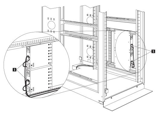
Figure 50. Connecting and routing the line cord
