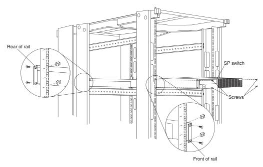
Figure 36. Installing an SP switch
