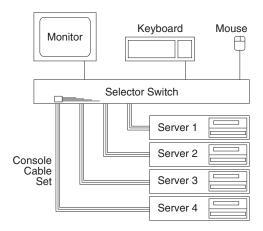
Figure 76. Single selector switch
