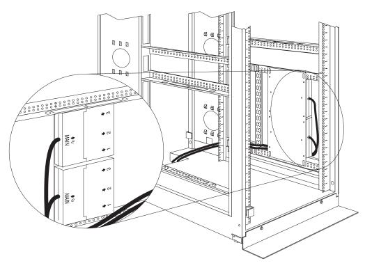
Figure 60. Routing the fixed line cords
