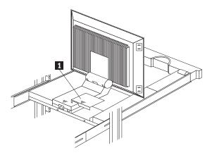
Figure 87. Routing the keyboard cable
