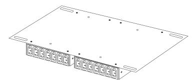
Figure 44. Installing a second Rack PDU
