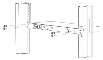
Figure 30. Power distribution horizontal installation
