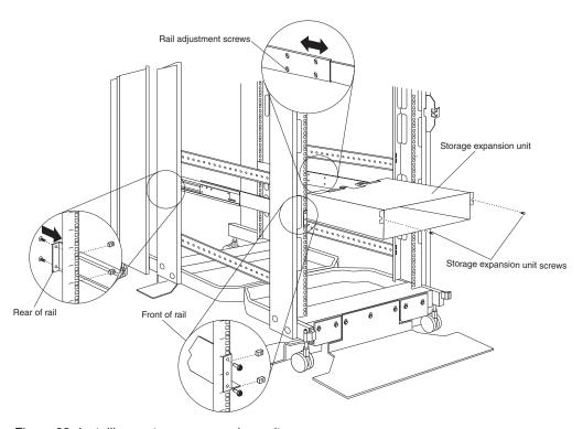
Figure 33. Installing a storage expansion unit
