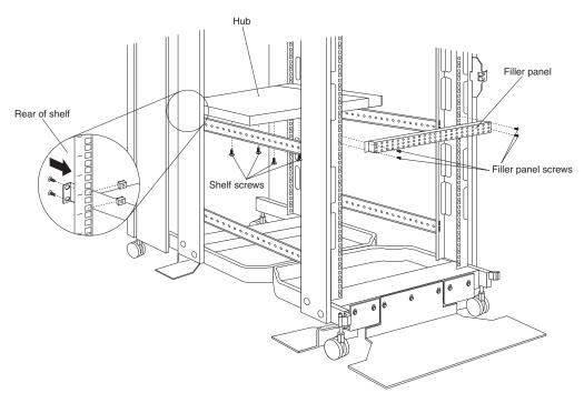
Figure 35. Installing a Fibre Channel hub
