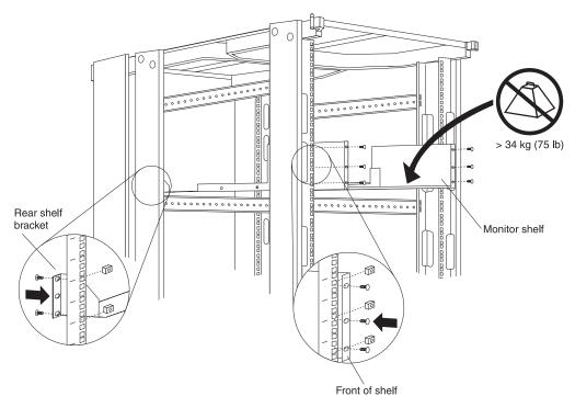
Figure 40. Installing a monitor shelf
