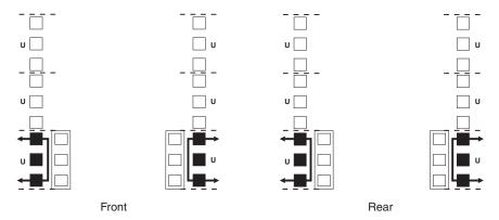
13. Slide the tray all the way inward; then, with one person at the front of the rack cabinet, and one person at the rear of the rack cabinet, carefully tilt the flat panel monitor and keyboard tray at an angle and slide it into the rack cabinet.
