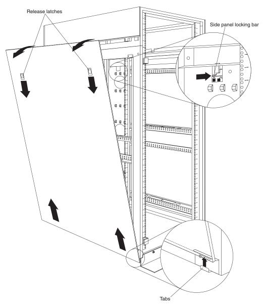
Figure 19. Removing the rack side panels
