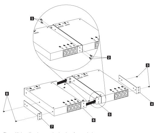
Figure 67. Installing the mounting brackets for two devices
