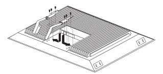
Figure 82. Installing the hinges on the flat panel monitor
