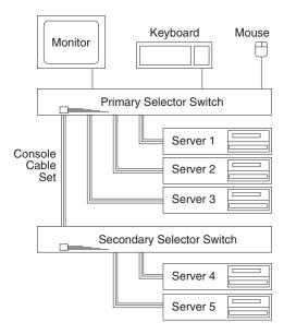
Figure 77. Multiple selector switch
