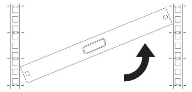
14. Adjust the rear slide-rail brackets to fit the depth of your rack cabinet; then, attach the brackets to the rack cabinet using four screws from the miscellaneous hardware kit.
