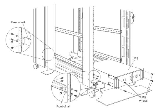
Figure 28. Installing a UPS
