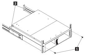
8. Tighten the rear screws 2.
