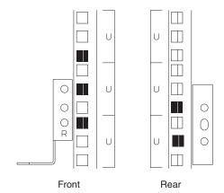
Note: Use clip nuts if your rack has circular holes. If your rack has square holes, you can use the rack-insertion tool or a flat-blade screwdriver to install cage nuts.
