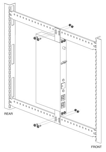
Figure 29. Power Distribution vertical installation
