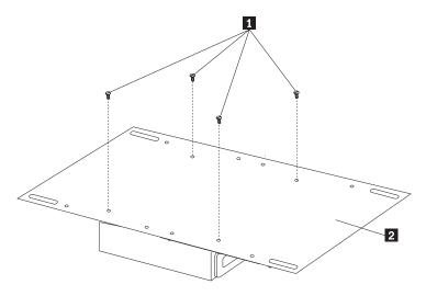
Figure 54. Installing the Rack PDU on the vertical mounting plate
