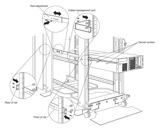
Figure 32. Installing a small server
