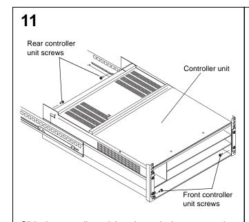
Slide the controller unit into the rack; then, secure the rear of the controller unit with two of the screws removed in step 10. Secure the front of the unit with the other two screws.
