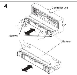
Loosen the four screws that secure the battery inside the controller unit; then, pull the battery out a few inches. Grasp both sides of the battery to remove it and save it for later reinstallation.
