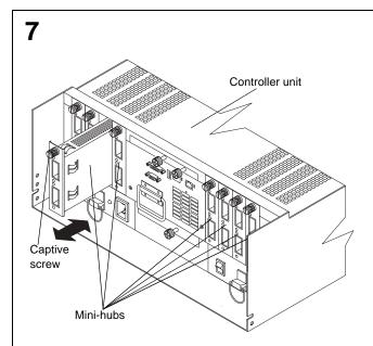
Loosen the captive screw on a mini-hub; then, grasp the screw to remove the mini-hub from the controller unit. Repeat step **7** for each mini-hub.
