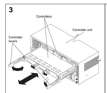
Unlock and open the controller levers; then, use the levers to pull the controller out slightly. Grasp both sides of the controller to remove and save it for later reinstallation. Repeat step 3 for each controller.
