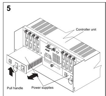
Using the pull handle on a power supply, lift up and pull to release the power supply; then, slide the power supply out and save it for later reinstallation. Repeat step **5** for each power supply.
