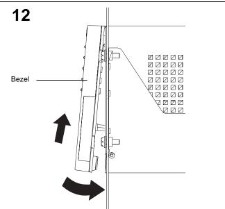
Reverse step 2 through step 7 to reinstall all of the devices that you removed; then, reinstall the bezel by sliding the top edge under the lip on the controller unit. Push the bezel bottom until it snaps into place.
