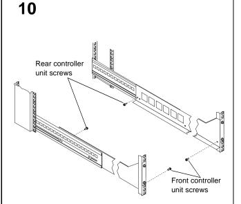
Remove the front and rear controller unit screws and save them to secure the controller unit to the rails.
