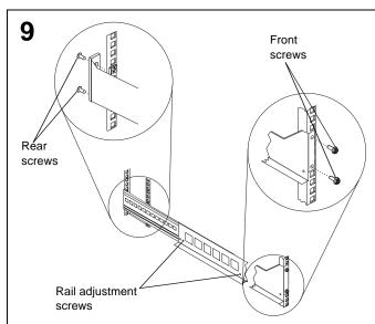
On the rail marked **R**, loosen both screws on the inside of the rail; then, extend the rail outside the rear rack mounting flange. Hold the front of the rail against the outside of the rack mounting flange and loosely insert the two front screws; then, insert and tighten the two rear screws and adjustment screws. Repeat step **9** for the rail marked **L**.
