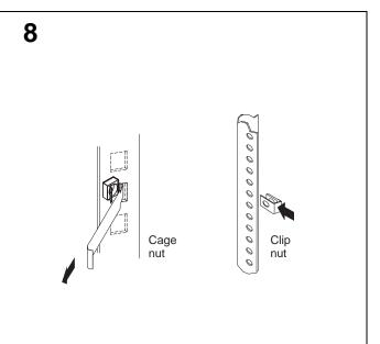
Insert cage nuts or slide clip nuts, as required for your rack, into all of the marked holes. Use the cage nut insertion tool or a flat-blade screwdriver to insert cage nuts.
