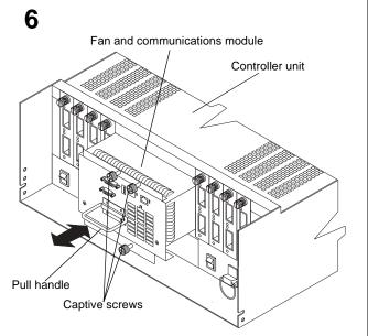
Loosen the three captive screws on the fan and communications module; then, grasp the pull handle and pull firmly to remove the module and save it for later reinstallation.
