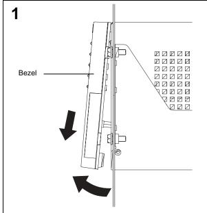
Carefully pull out the bottom of the bezel on the front of the controller unit to release the pins; then, slide the bezel downward and set it aside for later.
