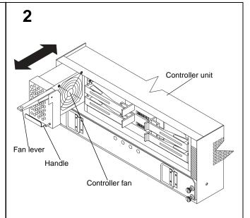
Pull up on the controller fan lever to unlock it; then, grasp the fan handle and pull out firmly to remove the fan and save it for later reinstallation.
