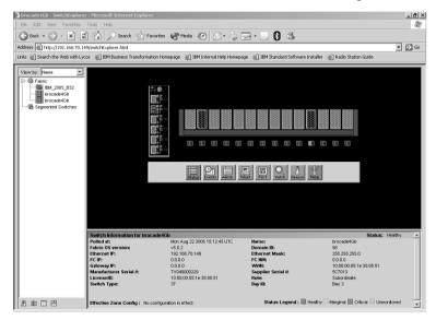
10. To perform switch-module administrative tasks, click Admin, and log in to the switch. In the User Name field, type the initial default user name, USERID. In the Password field, type the initial default password, PASSWORD (the sixth character is a zero, not the letter O). The user name and password are case sensitive.
