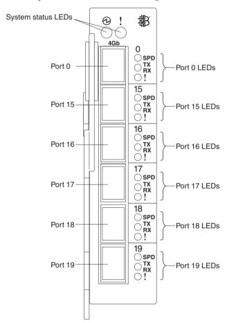
The switch-module information panel contains the following components:
