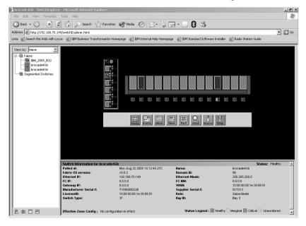
4. To perform switch-module administrative tasks, click **Admin**, and log in to the switch. In the **User Name** field, type the initial default user name, USERID. In the **Password** field, type the initial default password, PASSWORD (the sixth character is a zero, not the letter *O*). The user name and password are case sensitive.
