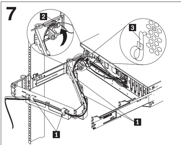
Attach the power cords and other cables to the rear of the server (including keyboard, monitor, and mouse, if required). Secure the cable-restraint bracket **2** to the slide rail.
