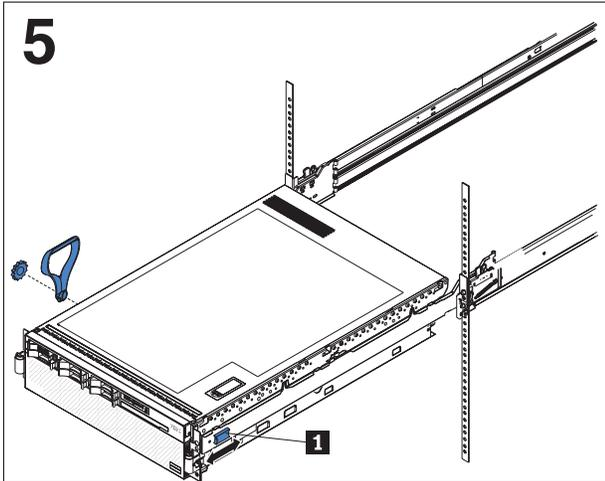
Remove the blue handles; then, slide the blue latches **1** on the slide rails in either direction and slide the server into the rack until it extends approximately 4 inches.
