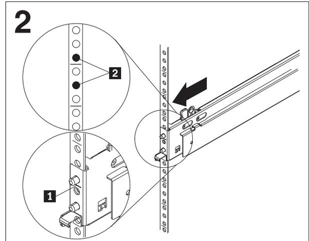
Align the left slide rail with the front mounting flange. Align the score mark **1** with the line between the top two 1-U installation positions. Push outward on the slide-rail latch to close the latch and secure the slide rail. Do the same for the right front slide rail. Align the slide rail with the rear mounting flange. Close the latches to secure the rear of both slide rails.
