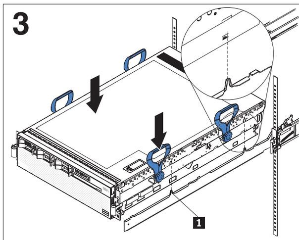
Extend the slide rails fully from the rack until the slide rails lock. Align the tabs on the slide rails **1** with the matching inserts on the server and lower the server onto the slide rails.
