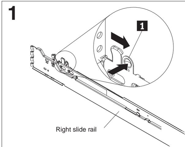
Push outward on the slide-rail latch **1**; then, pull the latch back to open the slide rail. The latch will catch to stay open. Open the other end of the slide rail; then, do the same for the other slide rail.
