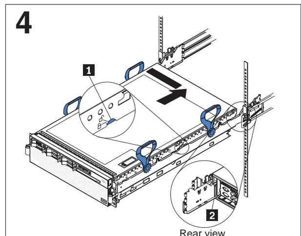
Carefully slide the server along the slide rails approximately one inch toward the rack to lock the server on the slide rails.
