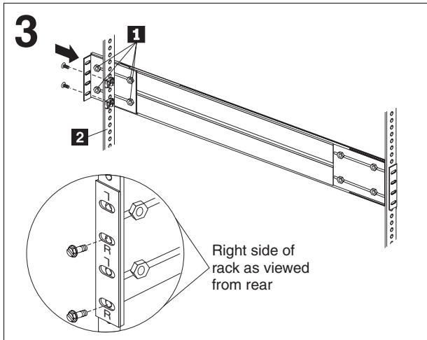
Align the slide rail to the rack-mounting flanges (front and rear). If it is necessary to adjust the length of the slide rail, loosen the nuts on the rear of the slide rail **1**; then, tighten the nuts. Insert and tighten two M6 screws to secure the slide rail to the rear-mounting flange **2**. Ensure that the rail is aligned vertically.
