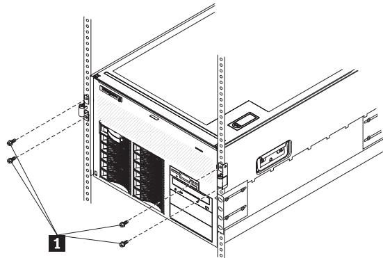
Insert the optional M6 screws **1** when moving the rack cabinet or if you install the rack cabinet in a vibration-prone area.
