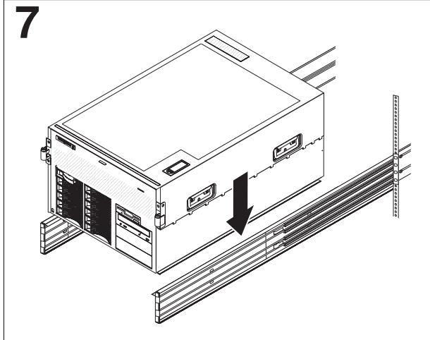
Extend both slide rails out of the rack cabinet until they lock. Align and slide the server onto the rails.
