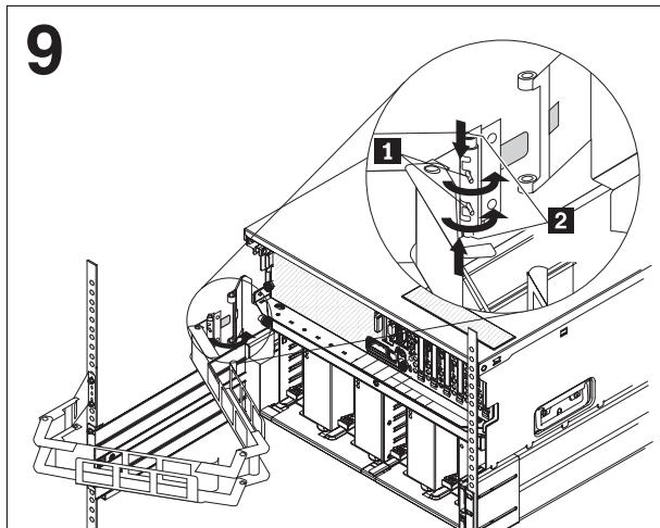
Using the handles **1** on the free end of the cable-management arm, retract the spring-loaded hinge pins **2**; then, rotate the handles to lock the pins in the retracted position.
