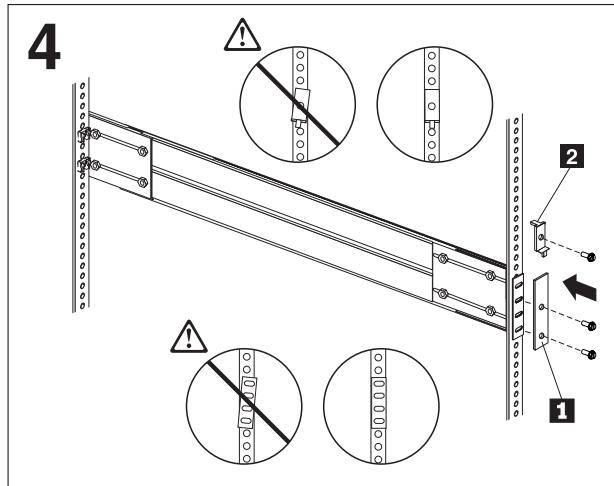
Position the cover plate **1** over the front of the slide rail; then, insert and tighten the two M6 screws. Ensure that the slide rail and cover plate are aligned vertically.
