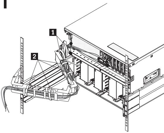
Attach the power cords and the keyboard, mouse, and USB cables to the server. Use two cable straps **1** to secure the cables to the cable-management-arm bracket.
