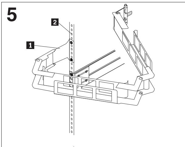
Position the cable-management arm **1** on the left rear rack-mounting flange **2** (as viewed from the back of the server) above the slide rail. Then, insert and tighten the two M6 screws to secure the arm of the flange.
