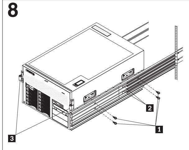
Secure the server to the rails with two M3.5 screws **1** on each side of the server; then, install the server cover.
