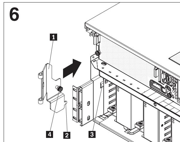
Attach the cable-management arm bracket **1** to the rear of the server by sliding tab **2** into slot **3**; then, tighten the captive screw **4**.
