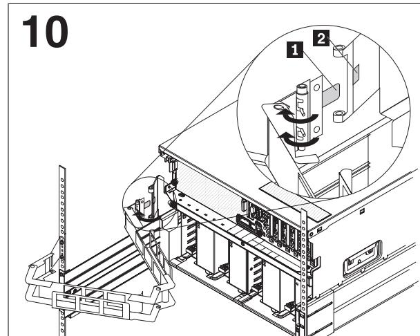
Slide the tab **1** on the cable-management arm into the slot **2** in the cable-management arm bracket; then, release the hinge pins into the holes in the bracket.
