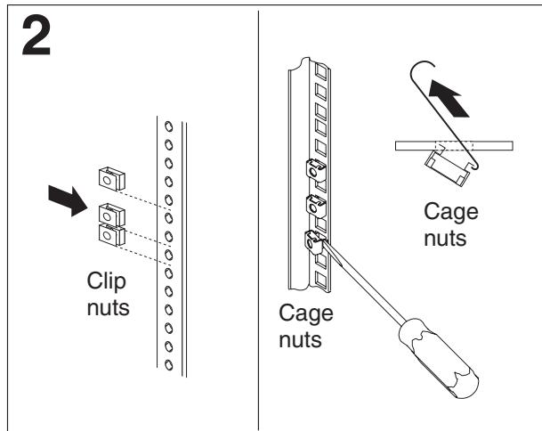
Use the arrows on the rack-mounting template to identify the locations to insert the clip nuts or cage nuts on the front and rear rack-mounting flanges **1**.
