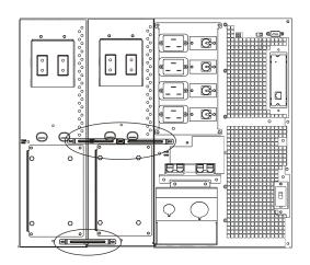
• Connect the green/yellow ground wire hanging from the battery pack to the TVSS screw on the uninterruptible power supply. For multiple battery packs, connect the wire to the TVSS screw on the nearest battery pack.
