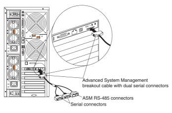
The ASM breakout cable with dual serial connectors also connects the Remote Supervisor Adapter II to the ASM interconnect network through the ASM RS-485 connector or to a modem through the serial connector.
