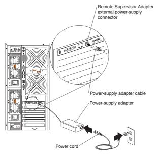
The following illustration shows the location of the power-supply connector on a Remote Supervisor Adapter II that is installed in a rack-mounted server.
