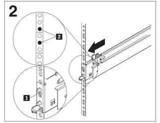
Align the left slide rail with the front mounting flange. Align the score mark with the line between the top two 1-U installation positions. Push outward on the slide-rail latch to close the latch and secure the slide rail. Do the same for the right front slide rail. Align the slide rail with the rear mounting flange. Close the latches to secure the rear of both slide rails.
