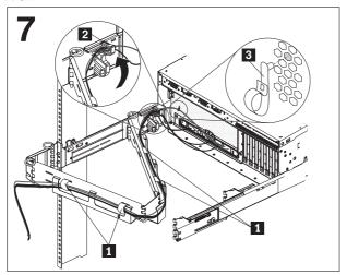
Attach the power cords and other cables to the rear of the server (including keyboard, monitor, and mouse, if required). Secure the cable-restraint bracket 2 to the slide rail.
