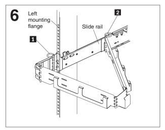
Attach the cable-management assembly to the rear of the slide rail using a hinge pin 1. Attach the free end of the cable-management assembly to the slide rail using the second hinge pin 2. Note: If you installed the cable-management-arm bracket in step 1, complete the installation of the cable management assembly.
