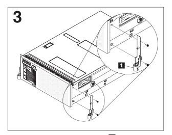
Install the release-latch brackets **1** . Insert a M3.5 flat-head screw in the top position and a M3.5x6 screw in the lower position of each bracket.
