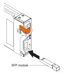
**Attention:** To avoid damage to the cable or the SFP module, make sure that you do not connect the fiber-optic cable *before* you install the SFP module.
