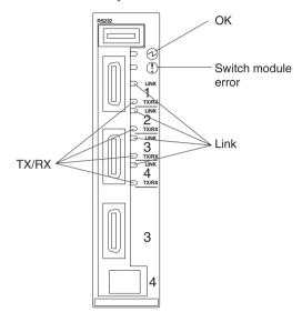
**Note:** An amber LED is lit when a system error or event has occurred. To identify the error or event, check the management module event log. For additional information, see Chapter 8, "Solving problems," on page 39.
