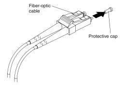
2. Gently slide the fiber-optic cable into the XFP module until it clicks into place.
