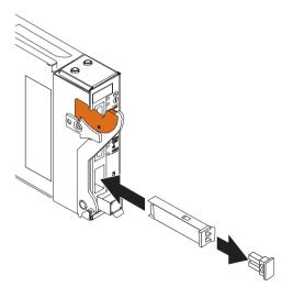
**Attention:** To avoid damage to the cable or the XFP module, make sure that you do not connect the fiber-optic cable *before* you install the XFP module.
