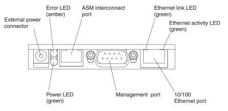
• External power connector - This cable connector is used to connect an external power supply to the Remote Supervisor Adapter.
