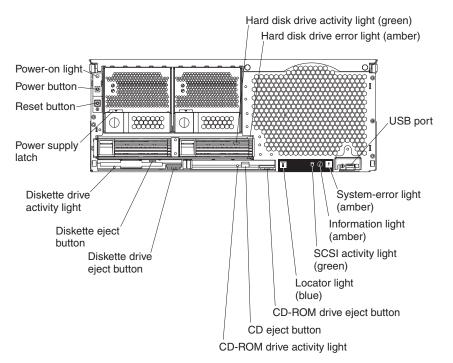
**Power-on light:** This green light turns on and stays on when you turn on your server, and it blinks when the server is in Standby mode.
