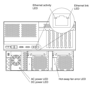
**Ethernet activity LED:** When this green LED is on, there is activity between the server and the network. The Ethernet activity LED is located on the Ethernet (RJ-45) connector on the rear of the server.
