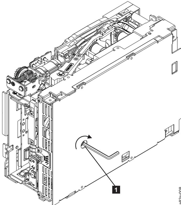
Figure 24. Using hex wrench to rewind tape into cartridge
