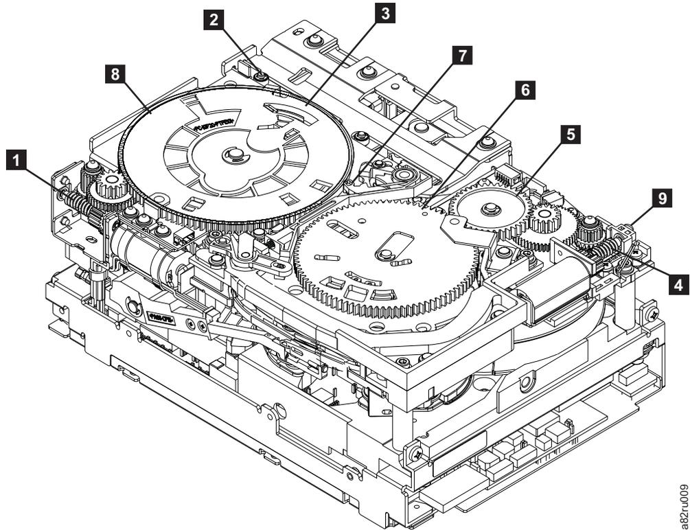
Figure 21. Drive with cover removed to reveal gear train.
