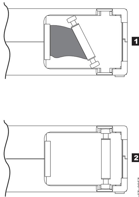
Figure 11. Leader pin in the incorrect and correct positions. The cartridge door is open and the leader pin is visible inside the cartridge.
