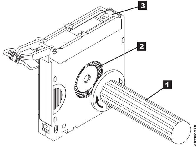
*Figure 16. Winding the tape out of the cartridge.* Turn the cartridge manual rewind tool clockwise to see the end of the tape, then turn it counterclockwise to bring the tape to the cartridge door.
