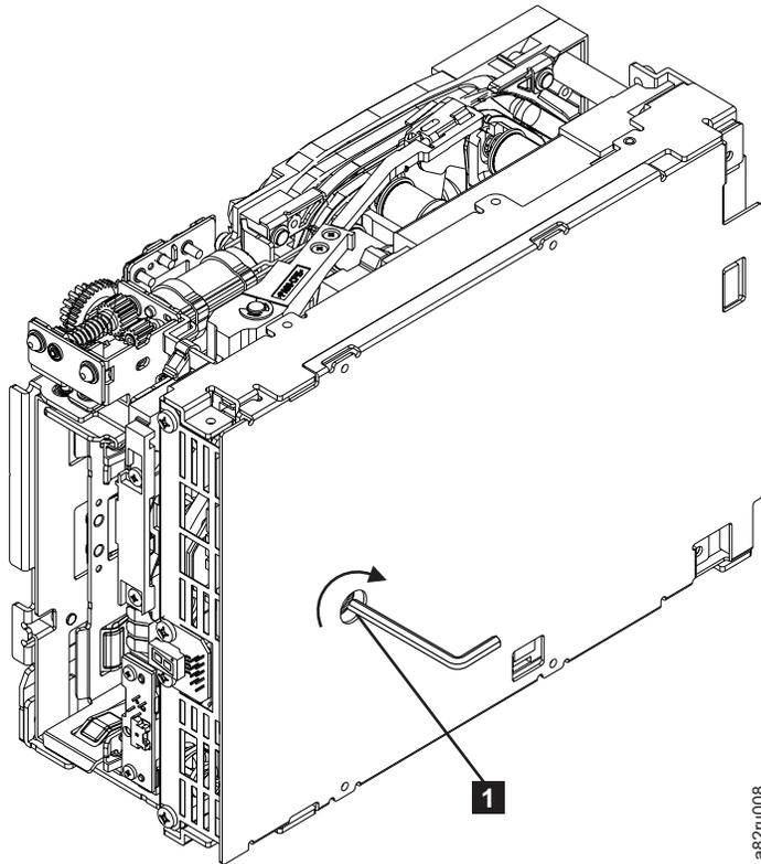
Figure 20. Using hex wrench to rewind tape into cartridge
