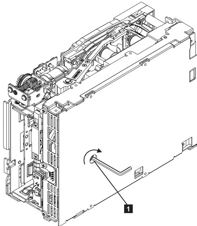
Figure 23. Using hex wrench to rewind tape into cartridge
