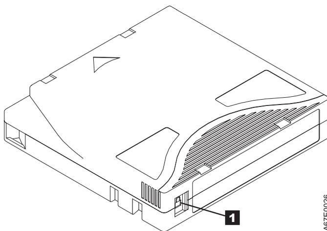
Figure 10. Setting the write-protect switch
