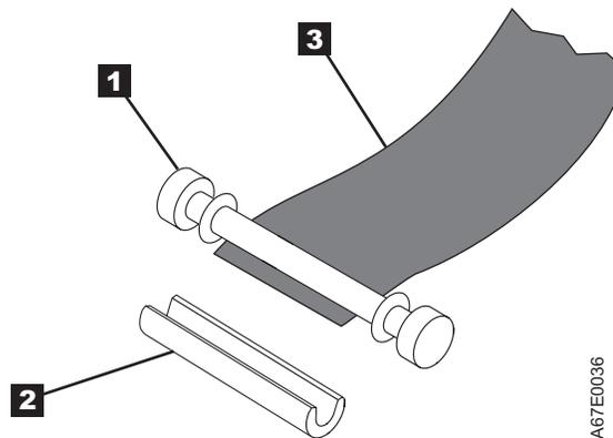
*Figure 17. Removing the C-clip from the leader pin.* Use your fingers to push the C-clip from the leader pin.
