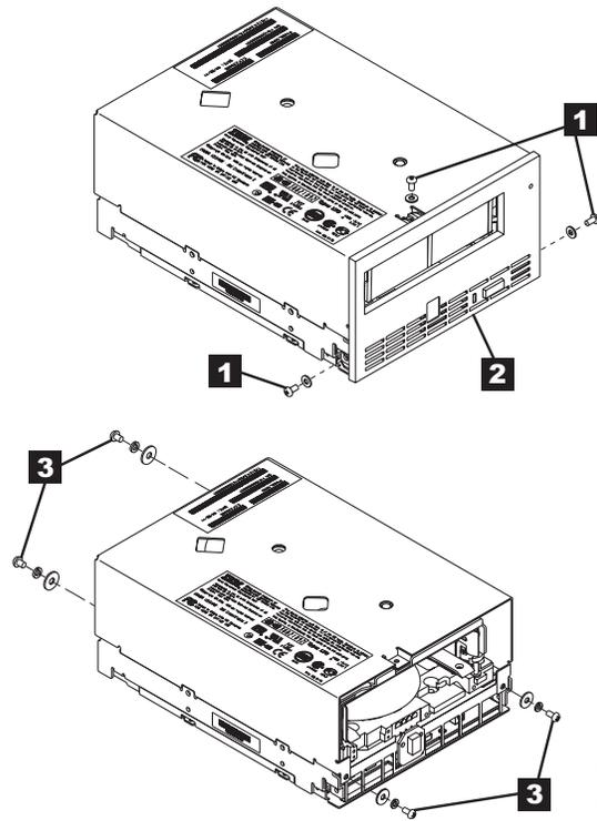
Figure 19. Removing the cover from the internal drive
