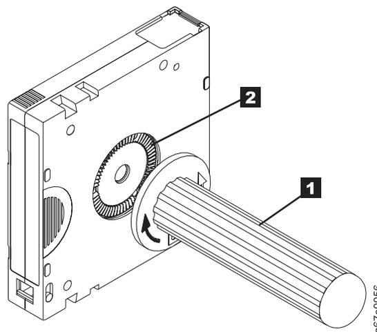
Figure 13. Rewinding the tape into the cartridge
