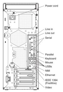
Depending on the video adapter that is installed in the computer and the monitor that you are using, you might have to use special video cables that convert signals or provide an additional connection point for dual-monitor capability. See the *User's Guide* on the IBM *IntelliStation Documentation* CD and the documentation that comes with the monitor for additional information.
