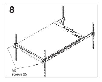
If you move the rack cabinet with the server installed, or if the rack cabinet is installed in a vibration-prone area, secure the server to the rack cabinet with one M6 screw in the top hole on each front rail bracket.
