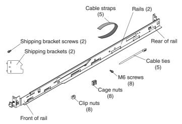
Use cage nuts for rack cabinets with square holes, use clip nuts for rack cabinets with round holes, and use your own rack screws for rack cabinets with tapped-holes. If your rack cabinet requires cage nuts, use a cage-nut-insertion tool or a flat-blade screwdriver to install them.
