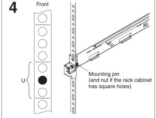
If the rack cabinet has round holes, remove the round nut from the mounting pin on the front of the rail. If the rack cabinet has tapped holes, use a Phillips screwdriver to unscrew and remove the mounting pin and nut assembly from the rail.
