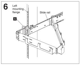
Attach the cable-management assembly to the rear of the slide rail using a hinge pin 1. Attach the free end of the cable-management assembly to the slide rail using a hinge pin.
