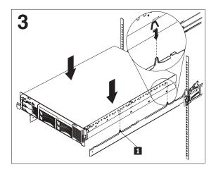
Extend the slide rails fully from the rack until the slide rails lock. Align the tabs on the slide rails **1** with the matching inserts on the server and lower the server on the slide rails.
