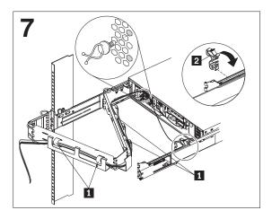
Attach the power cords and other cables to the rear of the server (including keyboard, monitor, and mouse, if required). Attach the power cords to the cable-restraint bracket **2**. Secure the cable-restraint bracket to the slide rail.
