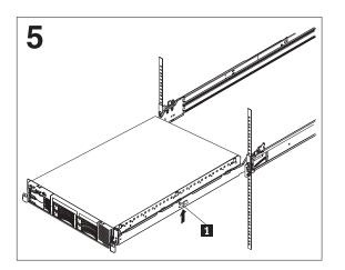
Lift the locking levers **1** on the slide rails and slide the server into the rack until it extends approximately 4 inches.
