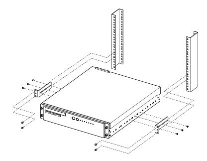
Multiple holes in the mounting bracket combined with multiple threaded holes in the chassis allow adjustment of the bracket on approximately ½-inch centers up to the practical limits of weight distribution. Attach the mounting brackets to the center three mounting holes (counting from the front or back, holes 4, 5, and 6) in the chassis using at least four of the six screws provided in the kit. Install the chassis in the rack using four rack screws (not provided in the rack mount kit).
