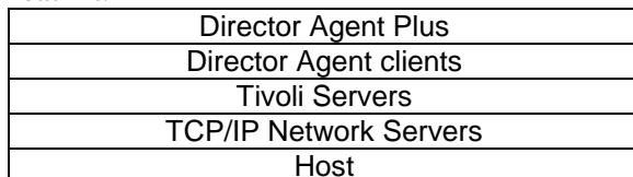
The most common reason for an interruption of service is a server failure or server hang, both of which can be cleared by stopping and restarting the server. Another common cause is a host problem that can be cleared by rebooting the host. When diagnosing a problem with Director Agent Plus for Tivoli, first confirm that layers of system services are operating correctly, in particular the Tivoli servers.
